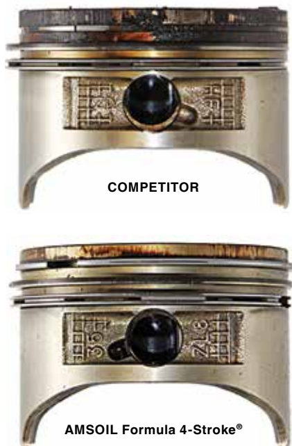
The pistons above were used in a proprietary AMSOIL severe-service four-stroke small-engine test in December 2014. The test, which runs 125 hours at 260°F, put AMSOIL Formula 4-Stroke Small Engine Oil up against a specialized competitive oil designed for commercial applications.
